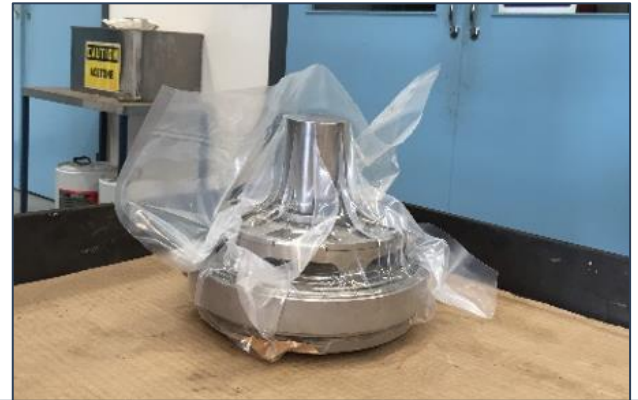
Vacuum-sealed wrapping for long term storage
