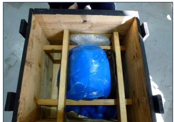
Volatile Corrosion Inhibitor (VCI) bags for alternate storage solutions
