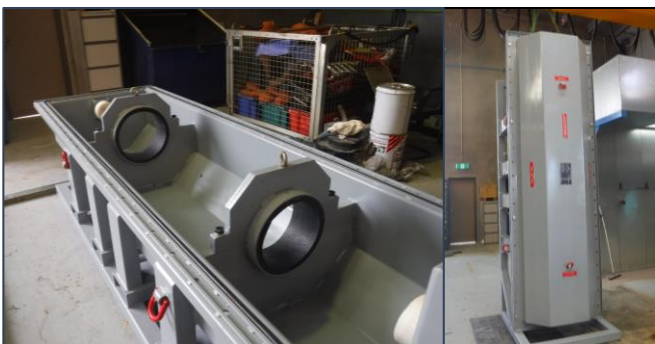
Nitrogen-purged rotor storage container for syngas turbine
