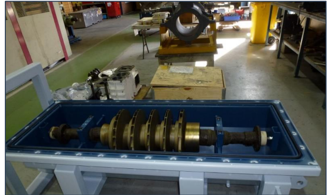
Nitrogen-purged rotor storage container for compressor
