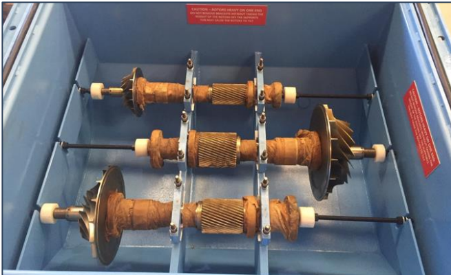
Integrally-geared compressor – Nitrogen-purged storage container
